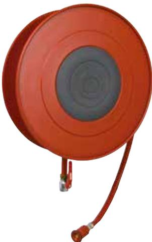
Fixed and swinging types for wall and recessed installation or base mounted with "Self-Standing" support. Carbon steel red painted reel in 535 mm or 600 mm drum diameter, supplied with grey plastic cover.
