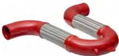
Seismic Joints are intermediary connection components used to absorb the unexpected random dynamic loads that may be originate from an earthquake and they are also used to remove the stress in the fire protection pipeline, by moving in six possible directions together with the building, in order to ensure the pipeline continue efficiency without any service interruption.
